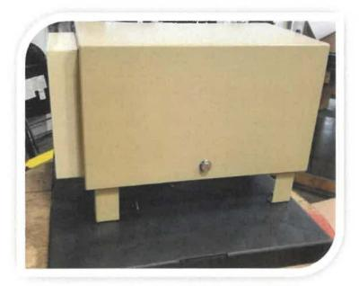
Soundproofing kit has been installed on single unit for testing.
